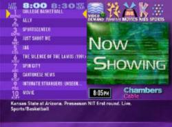
The viewer can then request one of these shows - usually movies – using their remote control. Their set-top box will then use its modem to send a request to the cable company for that show, and the computer at the head-end will start to play that program – but only for the viewer that requested it. And it adds a charge to the bill at the end of the month.
